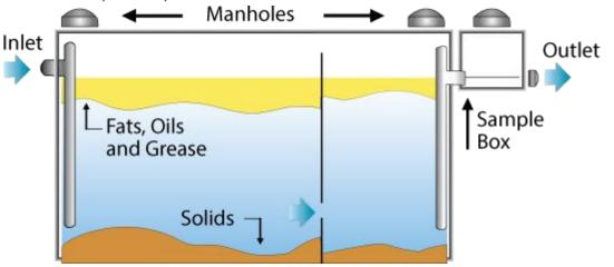
The grease and solids layers inside interceptors must not exceed 25% of the total volume. Service Authority inspectors will check FSEs' interceptors for compliance.
